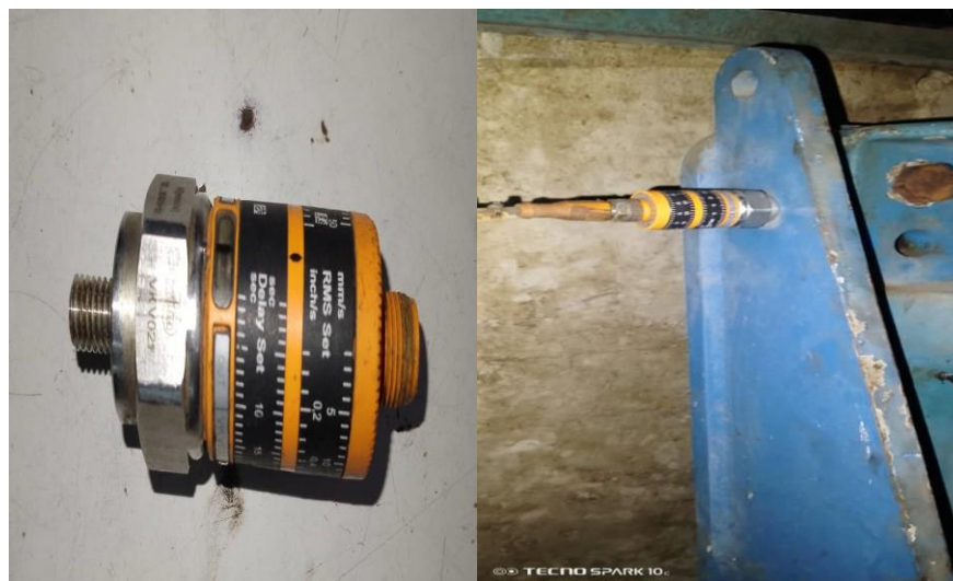
Plate 1: (a) Vibration monitoring sensor (VKV021), (b) VKV021 installed through PLC
